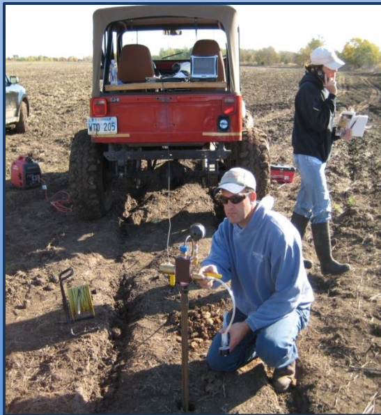
Performing a Pneumatic Slug Test
