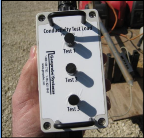
EC Test Load Used to Verify EC System is Working
